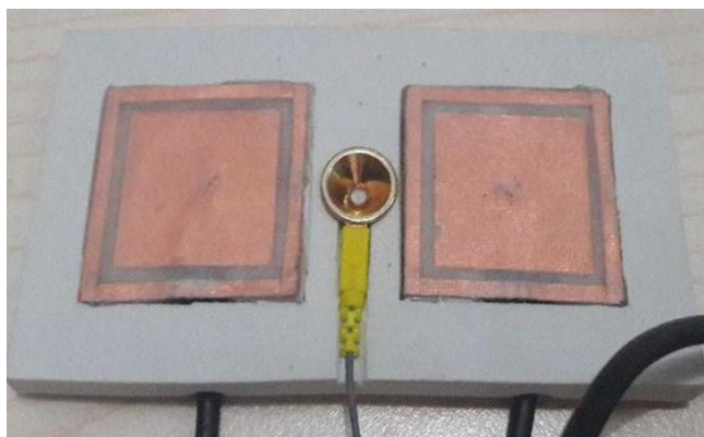
Fig 1: An Integrated Brain ECVT and EEG Sensor
